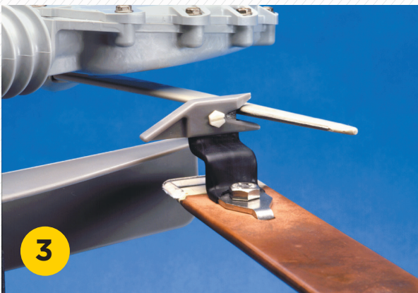
3 Current is fully transferred to the Interrupter and arc interruption is accomplished by thermal interaction of the arc on the specifically designed arc trailer and liner within the interrupter
